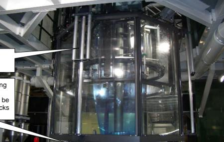
SB Lifting sys: 4 jacks / 1800mm stroke
